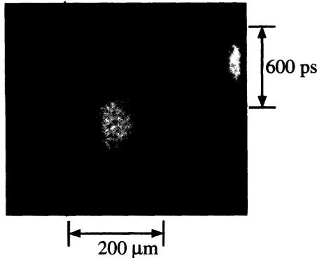
FIG. 1. Rear side shock breakthrough for a  $18 \mu\text{m}$  Al target. Optical smoothing is realized with RPP's giving a measured focal spot diameter FWHM= $106 \mu\text{m}$ . Time fiducial is on the right of the image.
