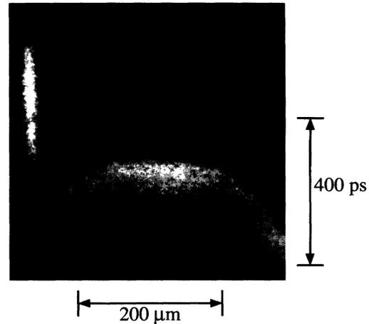
FIG. 2. Rear side shock breakthrough for a  $13.8 \mu\text{m}$  Al target. Optical smoothing is realized with PZP's giving a measured focal spot diameter FWHM= $400 \mu\text{m}$ . Time fiducial is on the left of the image.
