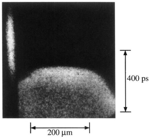
FIG. 2. Rear side shock breakthrough for a  $13.8 \mu\text{m}$  Al target. Optical smoothing is realized with PZP's giving a measured focal spot diameter FWHM= $400 \mu\text{m}$ . Time fiducial is on the left of the image.
