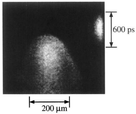
FIG. 1. Rear side shock breakthrough for a  $18 \mu\text{m}$  Al target. Optical smoothing is realized with RPP's giving a measured focal spot diameter FWHM= $106 \mu\text{m}$ . Time fiducial is on the right of the image.
