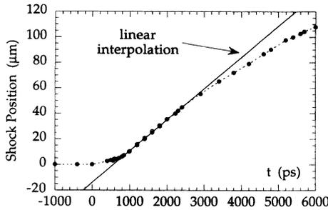
FIG. 3. Shock position as a function of time in Al target according to 1D code FILM simulations ( $I_L = 7 \times 10^{13}$  W/cm<sup>2</sup>, peaked at  $t = 1$  ns, FWHM=600 ps). The linear interpolation corresponds to a shock velocity  $D = 24$  μm/ns.
