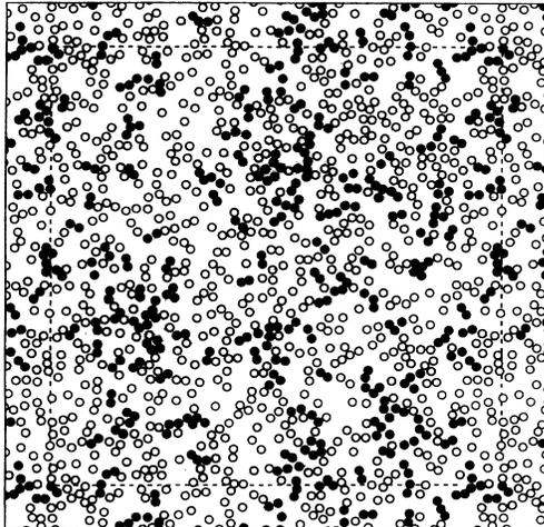
FIG. 4. The final ( $C/N=400$ ) “kinetic regime” configuration of  $N=1024$  inelastic disks with  $\nu=\frac{1}{4}$  and  $r=0.99$ . The solid disks are all the particles that participated in the final 200 collisions of this simulation.
