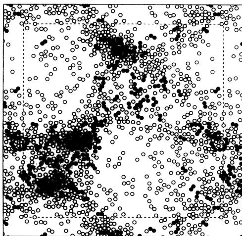
FIG. 5. The final ( $C/N=400$ ) “clustered regime” configuration of  $N=1024$  inelastic disks with  $\nu=\frac{1}{4}$  and  $r=0.8$ . The solid disks are all the particles that participated in the final 200 collisions of this simulation.
