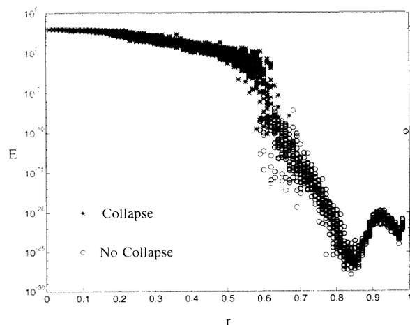
FIG. 7. The final energy in a suite of 600 simulations all with  $\nu=\frac{1}{4}$  and  $N=1024$ . At each of 100 values of  $r$  there are six realizations. The simulations that were stopped by collapse are indicated by an asterisk while those that ran till  $C/N=1500$  are indicated by an open circle.
