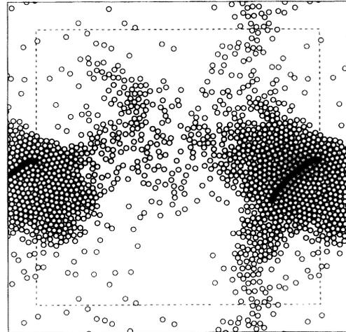
FIG. 6. The final ( $C/N=68.3$ ) “collapsed regime” configuration of  $N=1024$  inelastic disks with  $\nu=\frac{1}{4}$  and  $r=0.6$ . The solid disks are all the particles that participated in the final 200 collisions of this simulation.
