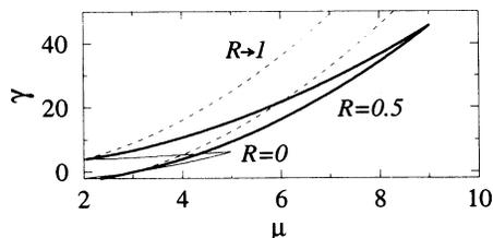
FIG. 1. Enhancement of control using ETDAS, illustrated with the parameters appearing in Eqs. (3) and (4). The region outlined in heavy lines produces a stable fixed point of the controlled map with  $R = 0.5$ . For comparison, the dashed lines (light lines) show the stable region for  $R \rightarrow 1$  ( $R = 0$ ).
