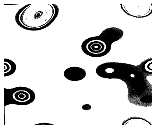
FIG. 4. (a) Integral reaction rate obtained for V_{ML}=0.825 l/ML > V_{ML}^* and p_{CO_e}=4.062 \cdot 10^{-5} Torr starting from a random initial phase distribution. The other parameters are the same as in Fig. 3. The snapshots of CO coverage correspond to time moments (b) t=4.5 s and (c) t=220.7 s; gray levels refer to coverage values.
