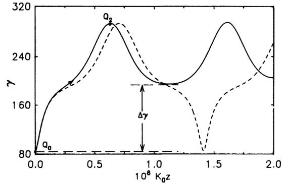
FIG. 4. Electron energy  $\gamma$  as a function of the traveling distance  $k_0 z$ . The electron motion states referred to are the same as those in Fig. 3. The solid line shows the energy variation in the presence of electrostatic field, while the dotted line is for that in the absence of electrostatic field.  $\Delta\gamma$  designates the low limit of the net acceleration.
