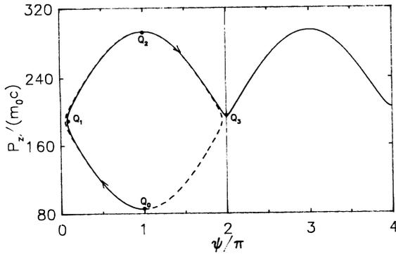
FIG. 3. Net acceleration mechanism for an electron moving in the  $\mathcal{D}_4$  region shown in Fig. 2. The electron is injected at  $\psi=\pi$  with initial  $\beta_z=0.999\,932$ . The parameters of the radiation field are the same as in Fig. 2. The dotted line shows the trajectory of the electron in the absence of static field. The solid line shows the same when  $qE_p=1\times 10^5$  eV/cm.
