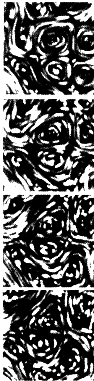
FIG. 5. Dipole evolution. The time interval between two successive images is 0.05 s. The dipole is a stable structure that can survey in the flow for a very long period of time.
