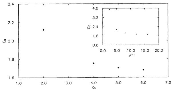
FIG. 3.  $C_D$  plotted against distance of obstacle center from inlet,  $X_0$ . Data are for  $f_i^0$  given by (1), and at  $Re = 48$ , with  $g = 1$ . The ratio  $\Lambda$  of obstacle diameter to system width is  $1/12$ . Inset:  $C_D$  plotted against the ratio  $\Lambda^{-1}$  of system width to obstacle diameter. Data are as for the main figure, but with  $X_0 = 4D$ .
