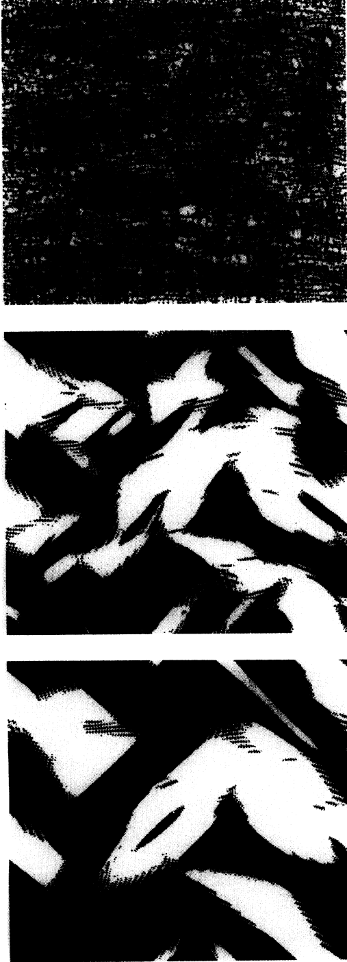
FIG. 6. The director field for r_0/D = 0.24 corresponding to the same times as in Fig. 1 ( t = 1600, 12800 , and 102400 ). The entire 512 \times 512 lattice is shown. The lower left quarter box corresponds to the 256 \times 256 region shown in Fig. 1. White denotes regions with \cos(2\theta) > 0 ( -\pi/2 < 2\theta < \pi/2 ) and black denotes \cos(2\theta) < 0 .
