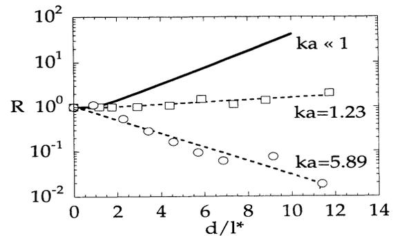
FIG. 3. Semilogarithmic plot of the ratio of the degrees of polarization  $R \equiv P_L/P_C$  as a function of  $d/l^*$ , for three values of  $ka$ . The solid line corresponds to the Rayleigh region ( $ka \ll 1$ ). The symbols indicate experimental data corresponding to measurements on suspensions of polystyrene latex spheres in water [0.22 ( $\square$ ) and 1.05 ( $\circ$ )  $\mu\text{m}$ ]. The dashed lines are a fit to Eq. (3).
