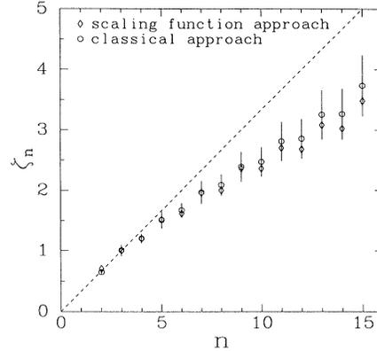
FIG. 2. Plot of the scaling exponents  $\zeta_n$  versus  $n$  computed using the scaling functions (diamonds) and the classical power-law fits (circles) [5]. The dashed line is the  $n/3$  prediction of Kolmogorov's 1941 theory.
