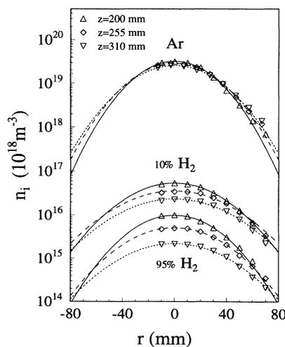
FIG. 3. Radial ion-density profiles for Ar and Ar-H<sub>2</sub> mixtures. The arc current is 45 A and reactor pressure is 0.5 mbar in all cases. The y scale is now logarithmic.
