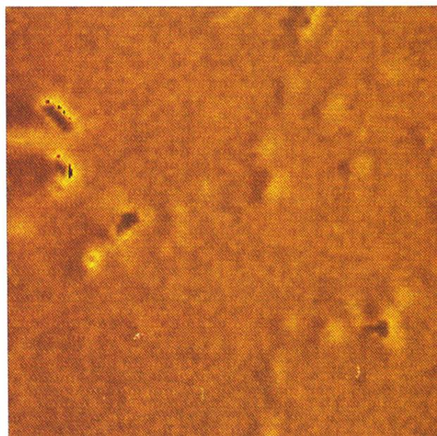
FIG. 5. (Top): photoelectron microimage similar to those of Fig. 1. (Bottom): the same area imaged by collecting photoelectrons at the energy corresponding to the K  $3p$  core level, and therefore reflecting the spatial distribution of potassium.
