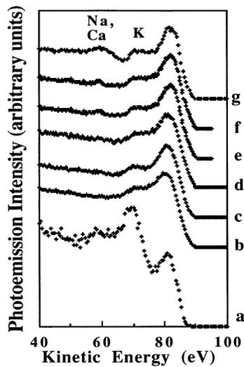
FIG. 2. A series of photoemission spectra taken with a photon energy of 95 eV in different  $1 \times 1\text{-}\mu\text{m}^2$  areas of two different neuron specimens. Curves a–e correspond to the first sample, and the remaining to the second sample. The probed area changes from curve to curve, always remaining on cell bodies. The labels identify spectral features due to specific elements.
