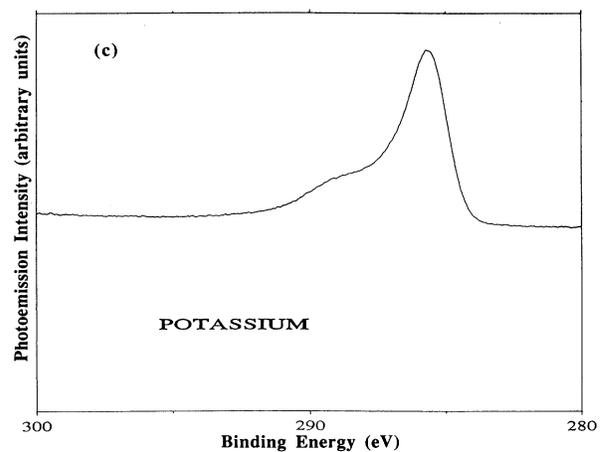
FIG. 4. Spectra taken with the Scienta ESCA-300 instrument in Lausanne, with Al  $K\alpha$  photons, over a macroscopic area of a specimen similar to those of Figs. 1–3. Curve a shows the spectral region of the Au valence electrons and of the (not observed) Ca  $3p$ , K  $3p$ , and Na  $2p$  electrons; curves b and c show the Ca and K  $2p$  core-level peaks.
