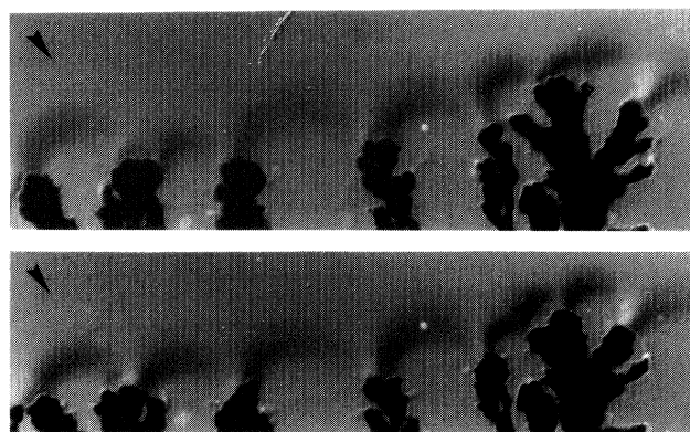
FIG. 17. Two consecutive images of the concentration gradient obtained with the interferential contrast (see text) on an almost steady growth. One should view the contrast on the pictures as the shadow of the concentration profile, with a spot light coming from the direction of the arrow. The concentration is 5 \times 10^{-2} \text{ mol l}^{-1} , a potential of 8 V was applied, the cell geometry is 0.1 mm \times 1 cm \times 1.5 cm (because of using constant potential in this experiment, the growth is not in the steady state).
