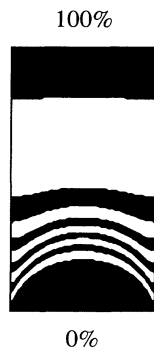
FIG. 12. Typical concentration map as given by the computation ( \mathcal{D}=5 \times 10^{-3} ). The alternate black and white stripes correspond to C_\infty/10 concentration intervals. The concentration is set to zero in the rear part of the branches (see the Appendix). Tips are at the bottom corners of the picture.
