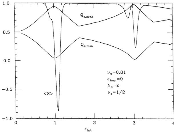
FIG. 2. The vertical spin vector and the perturbed spin tunes  $Q_{s,\max(\min)}$  obtained from a numerical tracking calculation at intrinsic resonance  $\nu_z = 0.81$  is plotted as a function of the resonance strength. Note that the perturbed spin tune covers the entire tune space at  $\epsilon = 1, 3$ .
