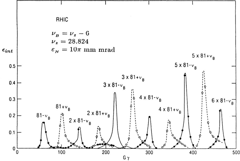
FIG. 12. The intrinsic resonance strengths calculated from a RHIC lattice. The expected resonance strength is about 0.45 at 250 GeV proton energy. The injection energy corresponds to  $G\gamma \approx 48$ , which happens to have a small intrinsic resonance strength.
