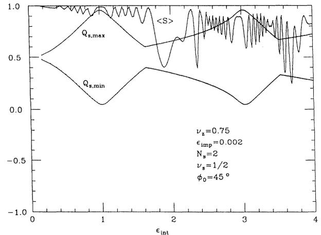
FIG. 7. The perturbed spin tune and the vertical spin component after passing through an intrinsic resonance at  $\nu_z = 3/4$  are shown as a function of the intrinsic resonance strength for  $\epsilon_{\text{imp}} = 0.002$ .
