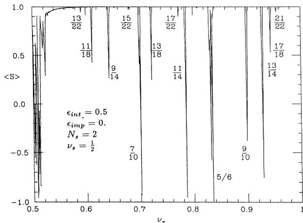
FIG. 1. The final vertical spin vector after passing through an intrinsic depolarization resonance with strength  $\epsilon_{int} = 0.5$  of an accelerator with two snakes is plotted as a function of the fractional part of the vertical betatron tune.
