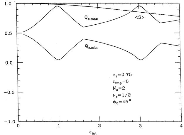
FIG. 5. The perturbed spin tune and the vertical spin component after passing through an intrinsic resonance at  $\nu_z = 3/4$  are shown as a function of the intrinsic resonance strength for  $\epsilon_{\text{imp}} = 0$ .
