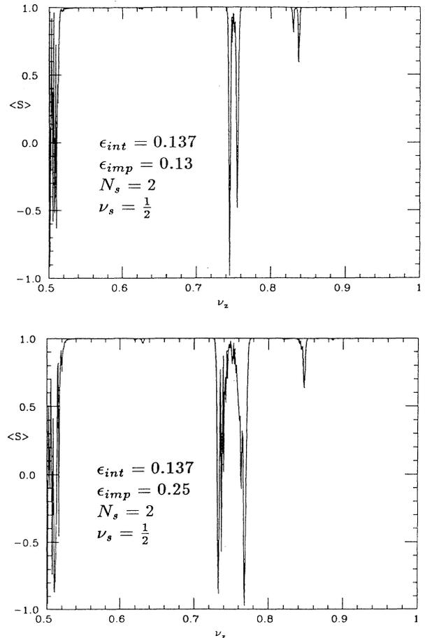
FIG. 9. The effect of the imperfection resonance on the snake resonances is shown for  $\epsilon_{imp} = 0.13$  (top) and  $\epsilon_{imp} = 0.25$  (bottom). Note that even-order snake resonances appear and each snake resonance splits into two resonance conditions due to the unperturbed spin tune of the imperfection resonance.
