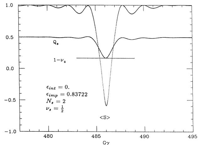
FIG. 4. The evolution of the vertical spin vector and the perturbed spin tune in the presence of an imperfection resonance at  $\epsilon = 0.83722$ . The betatron tune is chosen to satisfy Eq. (2.37) in order to demonstrate that the imperfection resonance does not contribute to the depolarization of a snake resonance.
