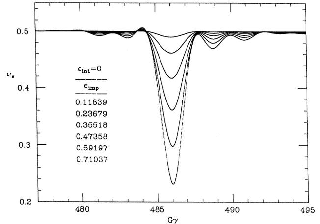
FIG. 3. The perturbed spin tune across imperfection resonances.
