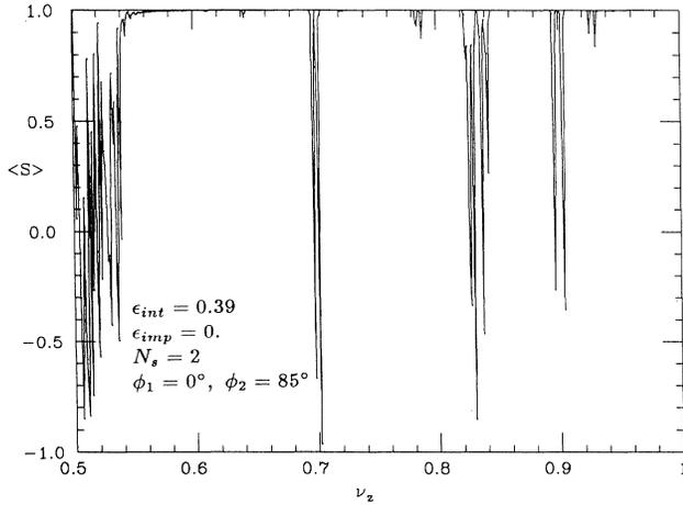
FIG. 11. The vertical spin vector after passing through an isolated intrinsic resonance for two snakes with spin axes angles with  $\phi_1 = 0^\circ$  and  $\phi_2 = 85^\circ$ . The spin tune is shifted from  $\frac{1}{2}$  by 0.028 without introducing imperfection resonances. Therefore each snake resonance is split into two without introducing even-order snake resonances.
