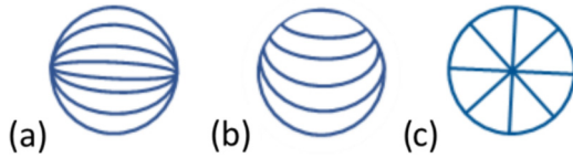
FIG. 1. Possible LC director configurations (director field lines) inside a droplet forming PDLC. (a) bipolar; (b) toroidal; (c) radial.
