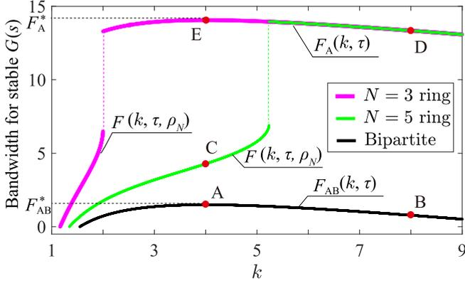
FIG. 8. Relationship between frequency bandwidth for stable  $G(s)$  and coupling strength  $k$  ( $\tau = 0.25$ ). Points A–D correspond to the parameters used in Figs. 6(a), 6(b), 7(a), and 7(b), respectively.
