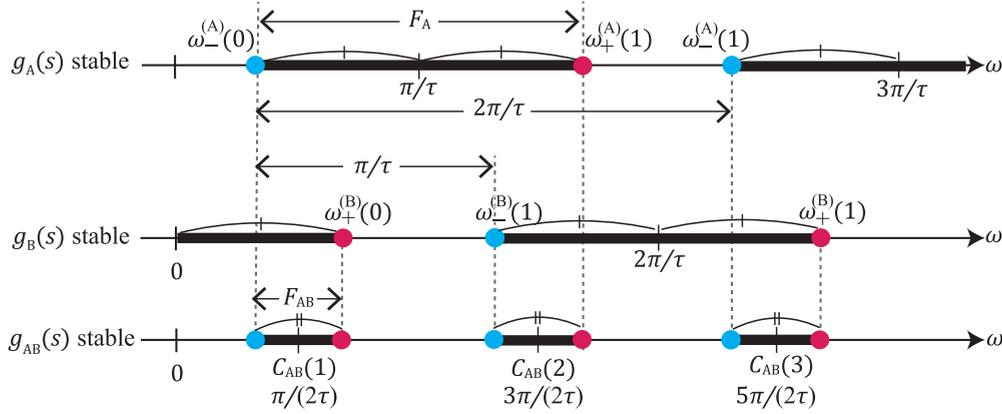
FIG. 4. Frequency band for stable  $g_A(s)$ ,  $g_B(s)$ , and  $g_{AB}(s)$  (i.e.,  $\Omega_A$ ,  $\Omega_B$ , and  $\Omega_{AB}$ , respectively).
