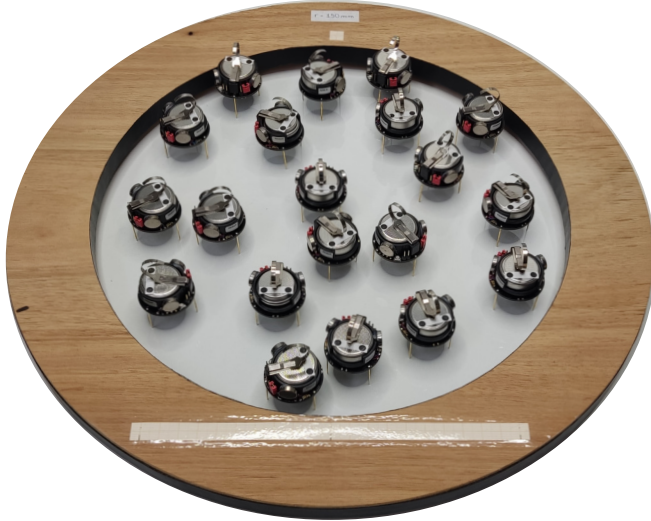
FIG. 2. Experimental setup. 20 Kilobots were positioned within a circular arena with a radius of 15 cm.
