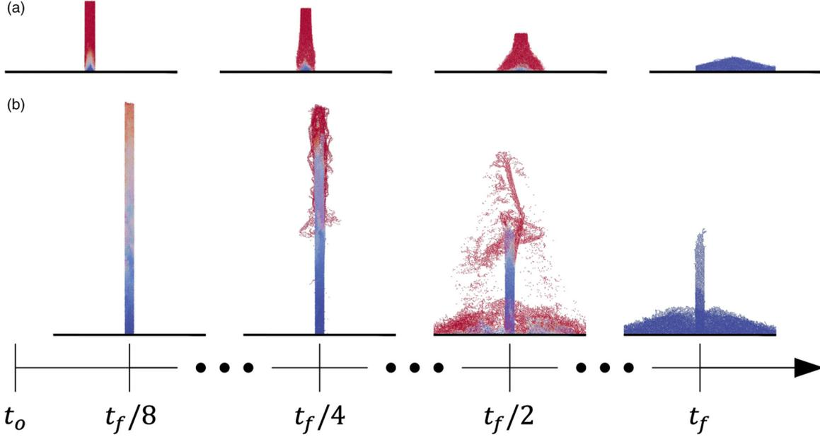
FIG. 10. Collapse sequence for a column with (a)  $N_a = 3$  arms and an initial height  $H_0/D = 66$  and (b) for  $N_a = 8$  and  $H_0/D = 240$ .  $t_f$  corresponds to the final time from which the heap is at rest. The color scale represents the particles' velocity.
