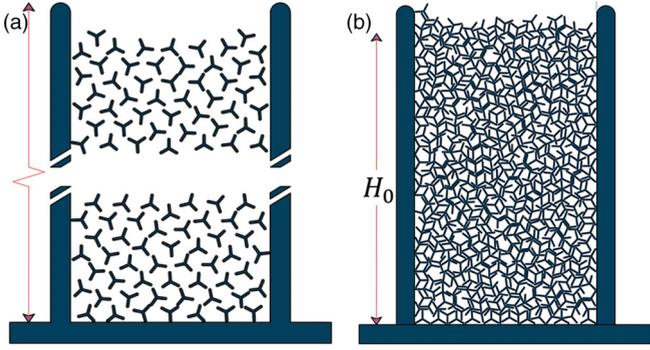
FIG. 2. Sample preparation: (a) Initial state of the sample construction, where  $N_p$  randomly oriented particles were initially laid on a triangular lattice (here for particles with three arms). (b) Final state, at the end of the gravity deposition phase; this pile served as an initial state for the stability test.
