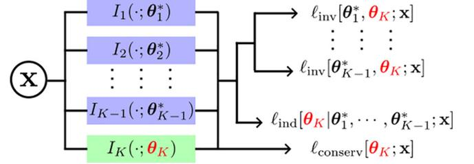
FIG. 2. Visual illustration of the learning framework. Previously learned conservation laws  $\{I_k(\cdot; \theta_k^*)\}_{k \in [K-1]}$  are fixed when training the  $K$ th conserved quantity  $I_K(\cdot; \theta_K)$ . The loss function  $\mathcal{L}_K(\theta_K; \mathcal{T})$  [Eq. (9)] is obtained by combining each loss over the training set  $\mathcal{T}$ .
