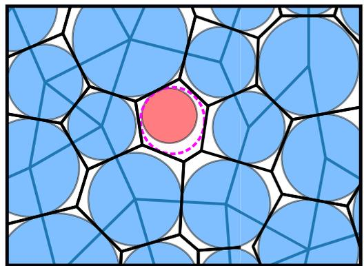
FIG. 9. The radical Voronoi diagram (black lines) is computed for a set of particles of different radii with contacts displayed as blue lines. All blue particles, labeled  $i$ , have  $M[R(\mathbf{r}_i)] = \bar{B}_{\sigma_i}(\mathbf{r}_i)$  and are thus stable. The red particle, which we will call 0 is a rattler, and its MIS is shown as a dashed magenta line. We see clearly that  $M[R(\mathbf{r}_0)] \neq \bar{B}_{\sigma_0}(\mathbf{r}_0)$
