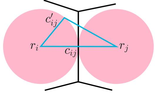
FIG. 6. The radical Voronoi diagram is shown between contacting particles  $i$  and  $j$  with contact point  $\mathbf{c}_{ij}$ . A second contact point between the two particles  $\mathbf{c}'_{ij}$  is assumed, so that we can show  $\mathbf{c}'_{ij} = \mathbf{c}_{ij}$  via the triangle inequality.
