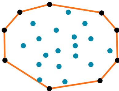
FIG. 3. Here we demonstrate the convex hull (orange) of a set of points. Points on the surface of the convex hull are colored black, while points not on the surface of the convex hull are in teal.
