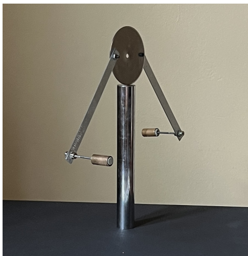
FIG. 2. Chiral rattleback built using a pizza cutter disk as a knife edge. The cylinder is for support only and is kept fixed.
