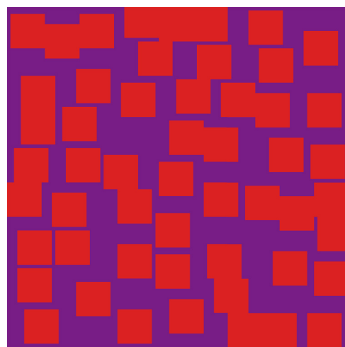
FIG. 13. Example of randomly filling a “big” square with the side L = 100 with “small” oriented squares having the side l = 10 . The small squares are randomly placed until the jamming limit is reached. In this example we could fit N = 54 small squares, corresponding to 0.54 filling, while the average value we obtained was slightly less than 0.56.
