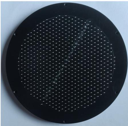
FIG. 3. Hexagonal grid of holes filled by steel spheres. The diameter of the disk is 150 mm; its thickness, including a lid, is 20 mm.
