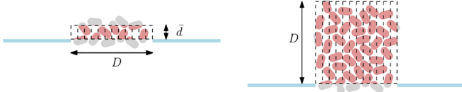
FIG. 11. Area of calculation for velocity profile (a) and packing fraction profile (b).
