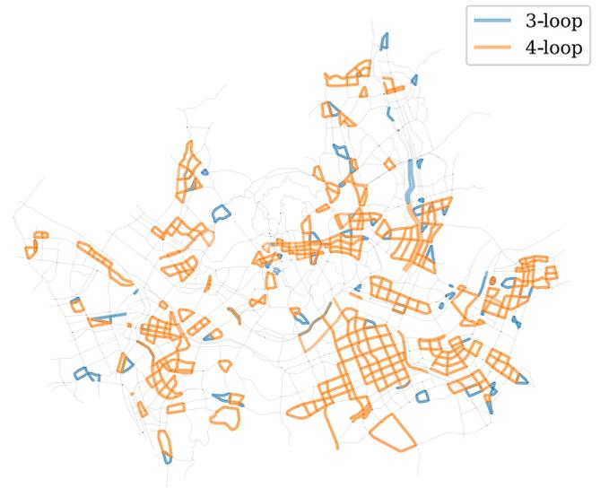
FIG. 9. Real-space representation of all possible 3- and 4-loops of congested flows in Seoul road network. The black thin line represents the underlying Seoul Road network. Blue and orange show all 3- and 4-loops of congested flows in the Seoul road network, respectively. Note that the bidirectional road might be overlapped in the real-space representation.
