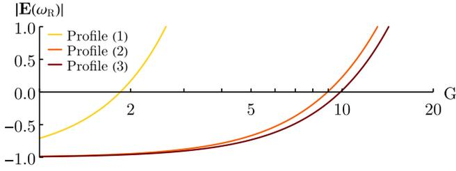
FIG. 3. Determinant of the dielectric matrix,  $|\mathbf{E}(\omega_R^{\text{crit}})|$ , as a function of  $G$ , for the profiles from Eqs. (4). For profile (1) [respectively, (2); (3)], the critical frequency is  $\omega_R^{\text{crit}} \simeq 1.047$  [respectively, 0; 0]. The value of  $G_{\text{crit}}$  is reached when  $|\mathbf{E}(\omega_R^{\text{crit}})|$  crosses zero.
