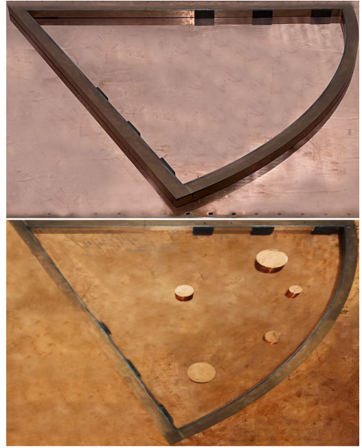
FIG. 1. Top: Cavity SB1 without lid. The microwave resonator is composed of a sector-shaped frame, shown in the photograph on top of a plate, which forms its bottom, and a top plate as lid. Bottom: Cavity SB2 without lid. It is obtained from SB1 by adding five copper disks of varying sizes and same height as the cavity. All parts are made from copper. To induce partial \mathcal{T} -invariance violation, three flat rectangular ferrite pieces (black rectangles) of length 50 mm, width 5 mm, and height 20 mm were attached symmetrically to both straight parts of the frame at a distance 425, 575, and 725 mm from the apex and magnetized with an external magnetic field of strength 169 mT.
