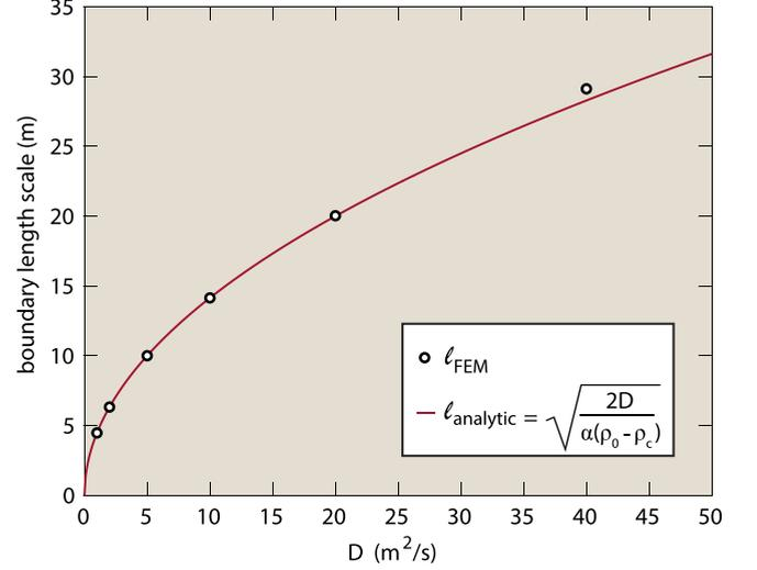
FIG. 6. Boundary layer thickness as a function of the neighbor coupling coefficient,  $D$ . A numerical result for the thickness of the boundary layer,  $\ell_{\text{FEM}}$ , was estimated by computing  $dv/dy$  at the wall and using the condition  $(dv/dy)\ell_{\text{FEM}} = v_{\text{pref}}$ , where  $v_{\text{pref}} = \sqrt{\alpha(\rho_0 - \rho_c)}/\beta$ . An analytical result for the thickness of the boundary layer,  $\ell_{\text{analytic}}$ , was calculated in Eqs. (74)–(77).
