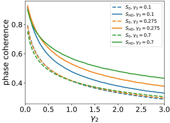
FIG. 4. Phase coherence generally vanishes with increasing  $\gamma_2$ , with fixed parameters  $\Delta = 0, E = 0.3, \theta = \pi/2$ . However, in the quantum regime, the presence of single-photon dissipation  $\gamma_3$  can boost phase coherence. Homodyne measurement greatly amplifies this boost in the quantum regime.
