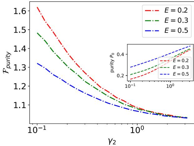
FIG. 2. Enhancement in purity of steady state due to homodyne measurement is always present but decays with increasing  $\gamma_2$ . (Inset) Purity scales approximately with  $\gamma_2^{1/3}$ . Fixed parameters:  $\Delta = 0$ ,  $\gamma_3 = 0.1$ ,  $\theta = \pi/2$ .
