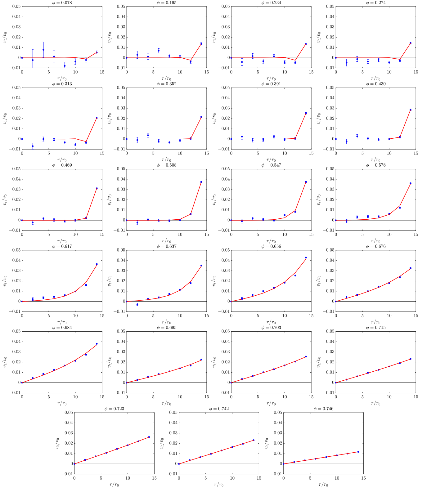
FIG. 9. The measured velocity profile for the various area fractions ranging from dilute gas to dense crystal and corresponding fits to the coarse-grained model.
