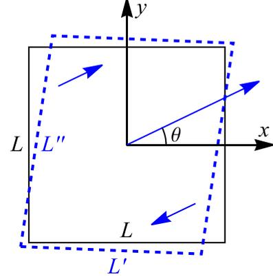
FIG. 1. Sketch of a simple shear deformation [Eq. (3)] applied to a square cell (with side length  $L$  and area  $A = L^2$ ) at an angle  $\theta$  to the  $x$  axis. The sides of the undeformed square cell (black solid lines) are aligned with the  $x$  and  $y$  axes. The deformed cell (blue dashed lines) has area  $A$  and side lengths  $L' = \|\bar{F}(L, 0)^T\|$  and  $L'' = \|\bar{F}(0, L)^T\|$ .
