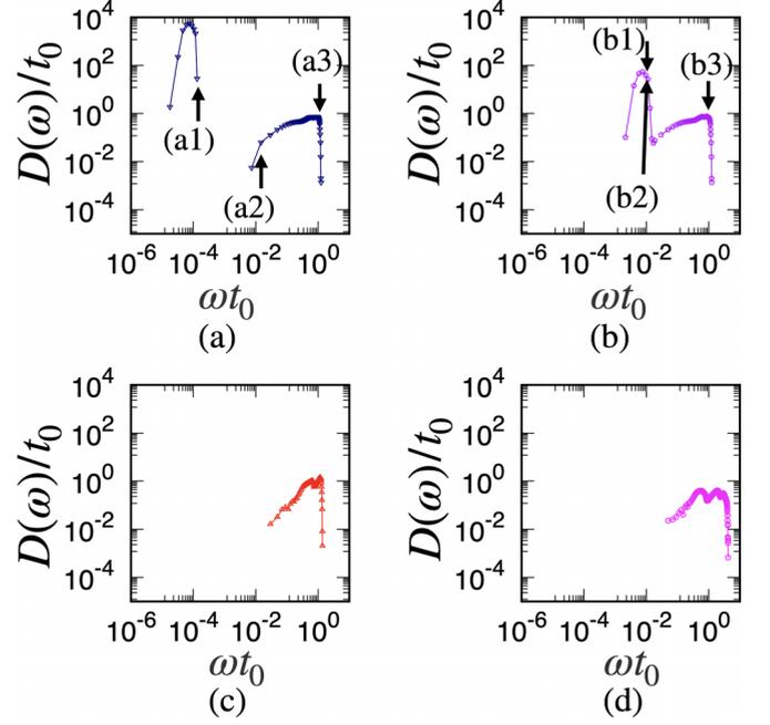
FIG. 9. Double logarithmic plots of  $D(\omega)$  against  $\omega t_0$  for  $\phi = 0.90$  at (a)  $k_T/k_N = 1.0 \times 10^{-8}$ , (b)  $1.0 \times 10^{-4}$ , (c) 1.0, and (d) 10.0. The eigenvalues of (a1), (a2), (a3), (b1), (b2), and (b3) in these figures correspond to Figs. 7(a1), 7(a2), 7(a3), 7(b1), 7(b2), and 7(b3), respectively. These figures are based on numerical results for  $N = 4096$ .
