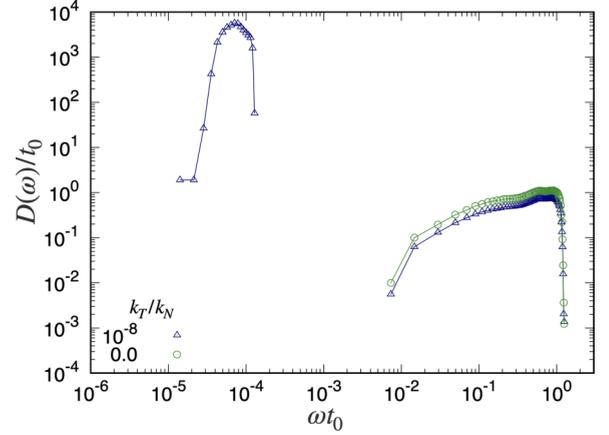
FIG. 11. Double logarithmic plots of  $D(\omega)/t_0$  vs  $\omega t_0$  with  $\phi = 0.90$ , where red circles are the DOS for frictional grains, while blue triangles are the DOS for frictionless grains. The figure is based on numerical results for  $N = 4096$ .
