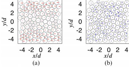
FIG. 2. Plots of (a) affine displacements and (b) nonaffine displacements of particles with  $\Delta\gamma = 1.0 \times 10^{-6}$ . Here, the magnitudes of the vectors are multiplied by (a)  $0.1\Delta\gamma^{-1}$  and (b) 1.3 for the visualization. These figures are based on numerical results for  $N = 128$ .
