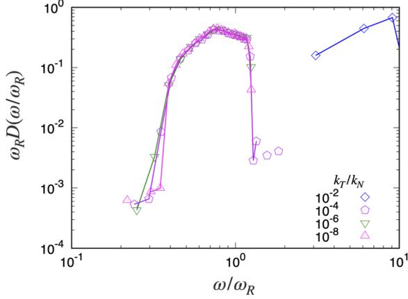
FIG. 10. Scaling plots of  $\omega_R D(\omega)$  versus  $\omega/\omega_R$  for  $\phi = 0.90$  and various  $k_T/k_N$  in  $0.1 < \omega/\omega_R < 10.0$ . The figure is based on numerical results for  $N = 4096$ .
