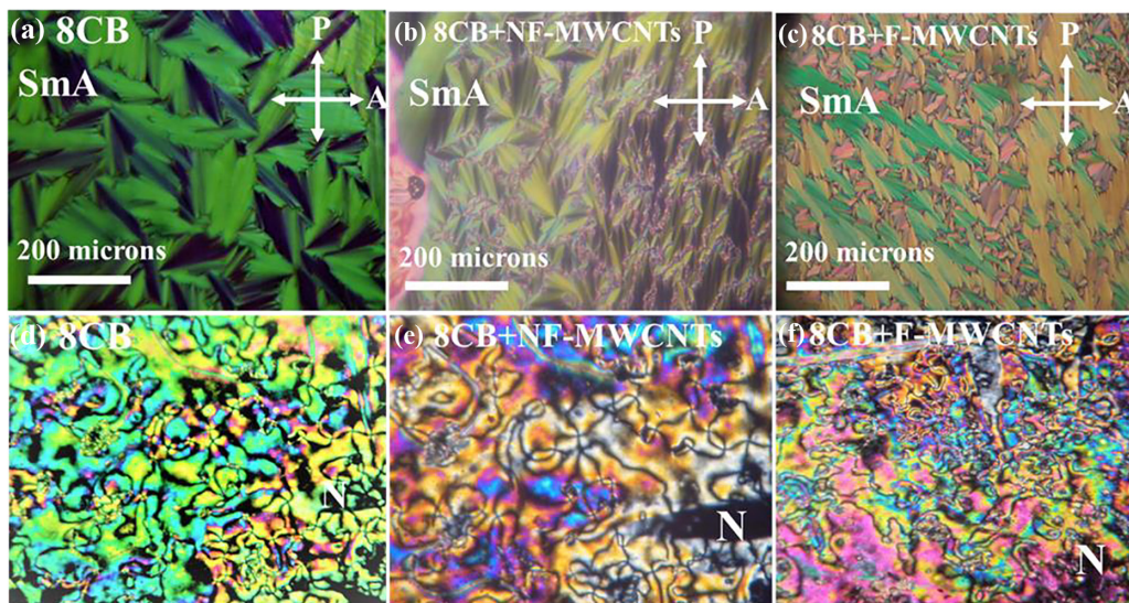
FIG. 2. Optical textures of (a) 8CB, (b) 8CB+NFMWCNTs, and (c) 8CB+FMWCNTs in the smectic A phase and (d) 8CB, (e) 8CB+NFMWCNTs, and (f) 8CB+FMWCNTs in the nematic phase under the cover slips.
