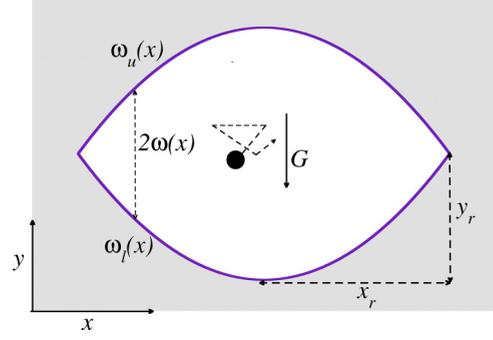
FIG. 1. Schematic illustration of two-dimensional monolobal confinement.  $\omega_u(x)$  and  $\omega_l(x)$  are the boundary functions of the confinement.  $x_r$  and  $y_r$  are characteristic length scales that describe the confinement boundary.  $\omega(x)$  is the local half-width at  $x$ .  $G$  denotes the external transverse force acting orthogonal to the feedback direction.
