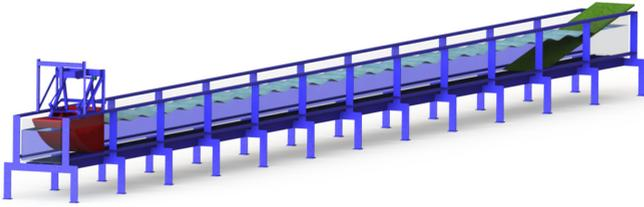
FIG. 2. The University of Sydney’s 30 m water wave tank comprising a piston-type wave maker and an artificial-grass wave absorbing beach installation.
