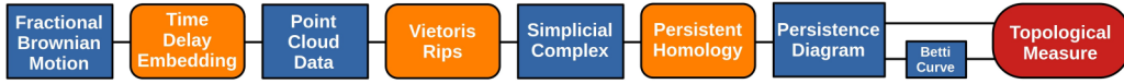
FIG. 4. The proposed pipeline in this paper: A synthetic fractional Brownian motion (fBm) time series is converted to a point cloud data (PCD) with the time-delay embedding (TDE) method. The evolution of homology groups of a simplicial complex mapped from the constructed point cloud data with the Vietoris-Rips (VR) method is calculated with the persistent homology (PH) technique and summarized as persistence pairs (PPs) in persistence diagrams (PDs). Finally, topological measures based on the persistence diagrams and Betti curves are computed.
