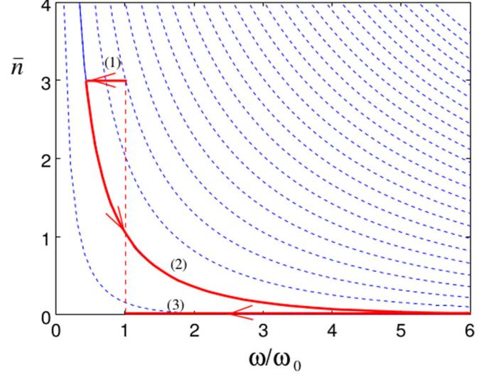
FIG. 7. Resetting the detectors with energy gap  $\hbar\omega$  (in units of  $\hbar\omega_0$ ): The evolution is marked by a red line in the  $(\omega, \bar{n}_D)$  plane. (1) Starting with  $\bar{n}_D = 3$ , adiabatically decrease  $\omega$  to reach the initial temperature. (2) Isothermally increase  $\omega$  to reach  $\bar{n}_D = 0$ . (3) Adiabatically return the frequency to its initial value. Broken blue lines are isotherms at various temperatures.
