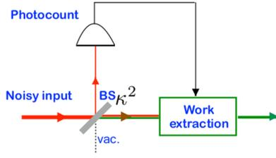
FIG. 1. Scheme of work extraction by quanta number detection (photocount) from a small fraction of a noisy input signal. The input is incident on a BS with high transmissivity  $\kappa^2$ , and the photocount is done on the reflected part. Work is extracted by unitary manipulation from the postmeasured transmitted part.
