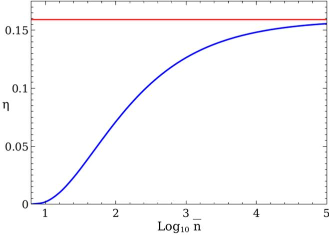
FIG. 8. Efficiency  $\eta = W/\hbar\omega\bar{n}$  plotted vs the mean number of input quanta  $\bar{n}$  for the scheme of sign measurement WOF. The red line represents the maximal  $\eta = 1/2\pi$ .
