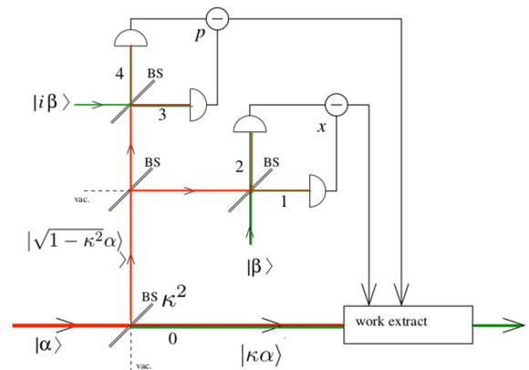
FIG. 4. Scheme of the setup for WOF by small-fraction homodyning: an unknown state (here labeled as coherent state  $|\alpha\rangle$ ) enters a beam splitter, which transmits a fraction  $\kappa^2$  of the input energy and reflects  $\sqrt{1 - \kappa^2}$ . On the reflected part, a homodyne measurement is performed to estimate the quadratures  $x$  and  $p$ .
