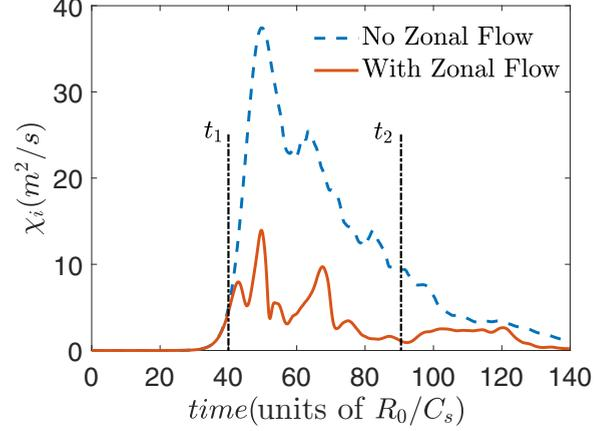
FIG. 1. Time history of turbulent ion thermal conductivities  $\chi_i$  at  $r = 0.45a$  with (solid) and without (dashed) zonal flows by using NLT with plasma parameters in Ref. [39].  $R_0$  and  $C_s = \sqrt{T_i/m_i}$  are the major radius in the magnetic axis and ion sound speed, respectively.
