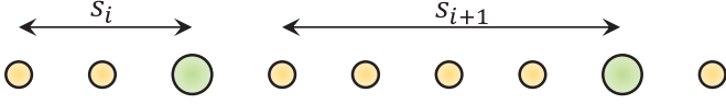
FIG. 1. Schematic illustration of the tight-binding chain. Small circles show the background lattice with zero on-site potential and the large circles are the impurities with on-site potential \lambda U . Here, s_i = 3 and s_{i+1} = 5 .
