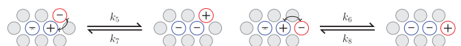
FIG. 5. All unique (up to rotational and translational symmetries) reversible reactions to destroy or produce clusters ( \ominus\ominus ) and ( \oplus\ominus ).
