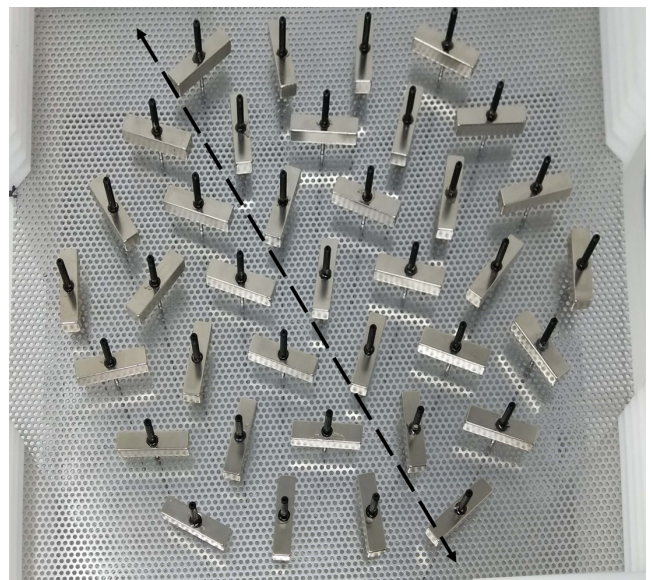
FIG. 4. One of the equilibrium configurations of rare-earth magnets in a triangular lattice.
