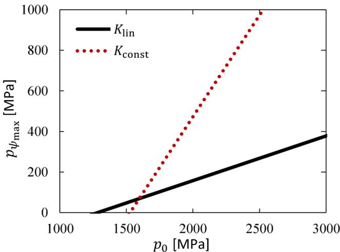
FIG. 9. Water: the course of critical pressure  $p_{\psi_{max}}$  for different values of inlet pressure  $p_0$  at 25 °C when considering  $K_{lin}$  and  $K_{const}$ .
