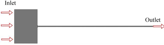
FIG. 4. Computational domain representing the flow of liquid from the reservoir to the nozzle.
