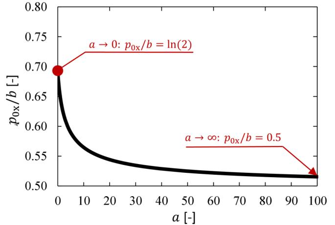
FIG. 10. The influence of parameter  $a$  in equation  $K_{lin} = ap + b$  on the value of the minimum pressure in the liquid reservoir when liquid-dynamic choking may occur.
