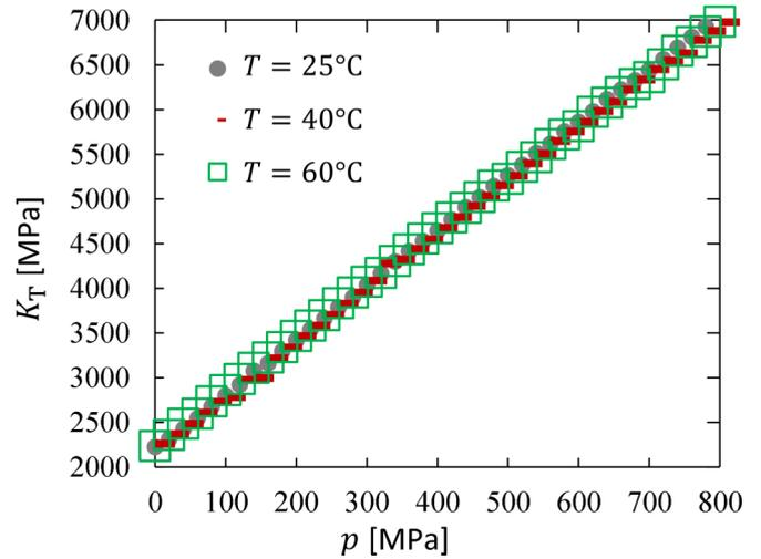
FIG. 7. Dependence of water bulk modulus on pressure at constant temperatures 25 °C, 40 °C, and 60 °C.
