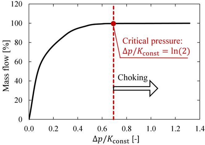
FIG. 6. The flow through the nozzle during an increase in the pressure difference between the inlet and outlet based on CFD analysis for the constant value of bulk modulus  $K_{const}$ .
