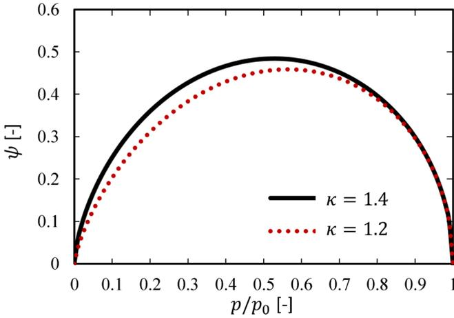
FIG. 1. Function  $\psi$  of an ideal gas for heat capacity ratio  $\kappa = 1.2$  and  $\kappa = 1.4$ .
