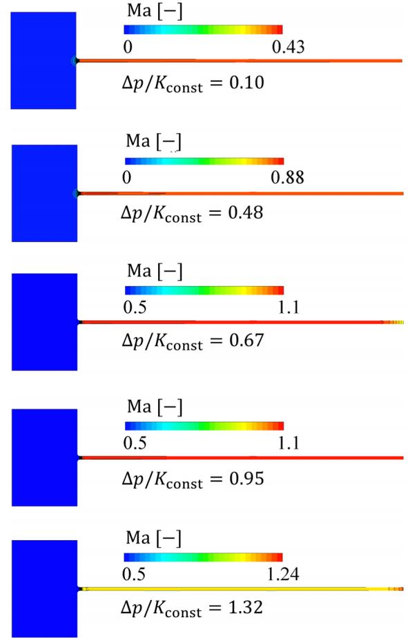
FIG. 5. Distribution of Mach number in the computational domain for selected values of ratio  $\Delta p/K_{\text{const}}$  obtained by CFD analysis performed for a constant bulk modulus.
