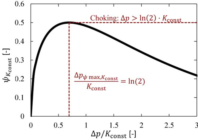
FIG. 2. The course of function  $\psi_{K_{\text{const}}}$  of a liquid with a constant bulk modulus  $K_{\text{const}}$ .
