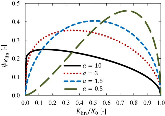
FIG. 3. The course of function  $\psi_{K_{lin}}$  of a liquid having linear dependence on the bulk modulus  $K_{lin}$  of pressure depends on the ratio of the bulk moduli  $K_{lin}/K_0$  for selected coefficients  $a$ .
