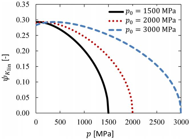
FIG. 8. The course of function  $\psi_{K_{lin}}$  on pressure  $p$  for water at 25 °C for three values of reservoir pressure  $p_0 = 1500, 2000,$  and  $3000$  MPa.
