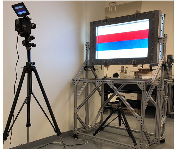
FIG. 1. Photograph of the Hele-Shaw device, filled with three liquid layers and air on top, before the overturn. The cell can be rotated about the pivot points at the center of the sides. The video camera is prefocused and mounted on a sturdy tripod.
