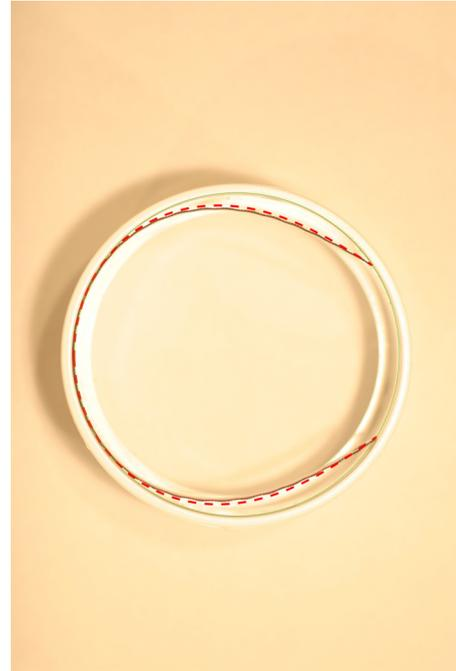
FIG. 5. A steel hacksaw blade of length  $L_H = 266 \text{ mm} = 4.97a$  confined within a PVC pipe coupling of diameter  $2a = 107 \text{ mm}$ . The dashed line is the fiber shape predicted in Secs. III and IV A.
