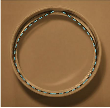
FIG. 6. As for Fig. 5, but with a hacksaw blade of length  $L_H = 315 \text{ mm} = 5.89a$ . The dashed line is the fiber shape predicted in Secs. III and IV A.
