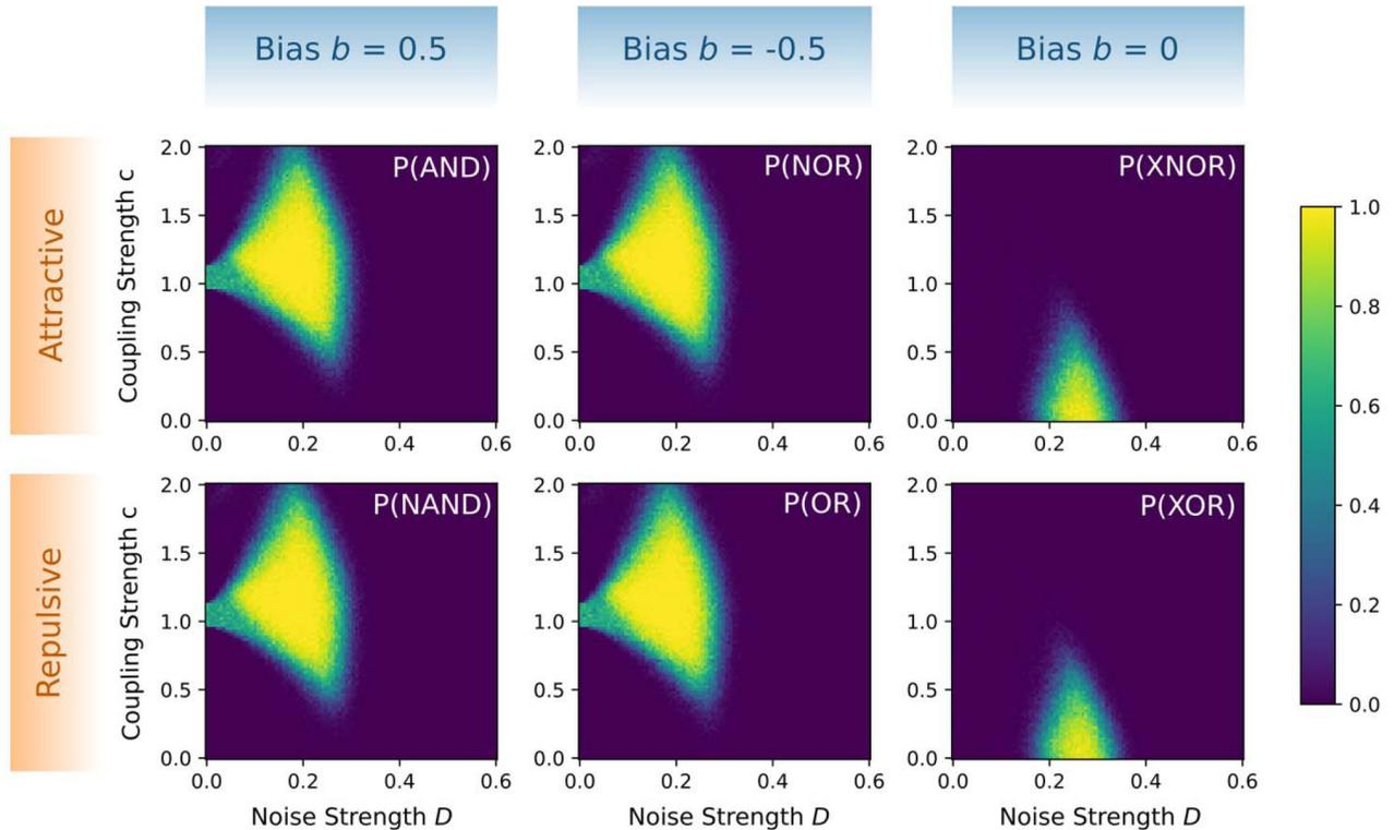
FIG. 5. Probability of obtaining reliable logic operations  $P(\text{logic})$  for all six fundamental logic operations [ $P(\text{AND})$ ,  $P(\text{NOR})$ , etc.] is plotted as a function of noise strength  $D$  and coupling strength  $c$ . The plots are made for both attractive and repulsive coupling schemes at three specific values of bias  $b$ , depicting broad regions in parameter space where all six logic operations are consistently obtained.
