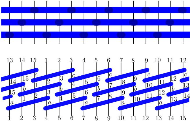
FIG. 19. Time step operator and its transfer matrix representation. This construction applies to models with four-site interactions where the outer two spins are control bits. These control bits are depicted as shaded circles in the figure above. An example is the folded XXZ model.
