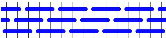
FIG. 12. A tightly packed quantum circuit with three-site gates. This network has periodicity 3 in both the space and time directions. Accordingly, we can prove the existence of commuting transfer matrices built from three rows.
