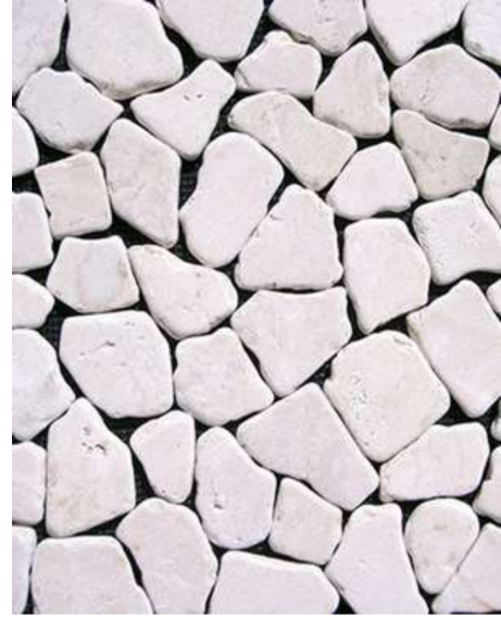
FIG. 5. An ensemble of stones that illustrates the basics of the dense solid-grain packing that is abundant in sedimentary rocks. As can be seen in the figure, the total porosity is lower than that of the random void model of Fig. 4, but as in that model, one can recognize that there are two groups of pores, those of the relatively wide aperture (the voids) and those of the narrow aperture (the throats). Note also that the pore spaces are connected [54,110], thus providing continuous conducting paths.
