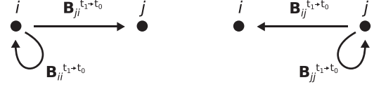
FIG. 4. Degenerate pitchforks composed of two nodes instead of three, i.e., when k = i or k = j respectively. Black dots represent network nodes, arrows symbolize directed temporal links.
