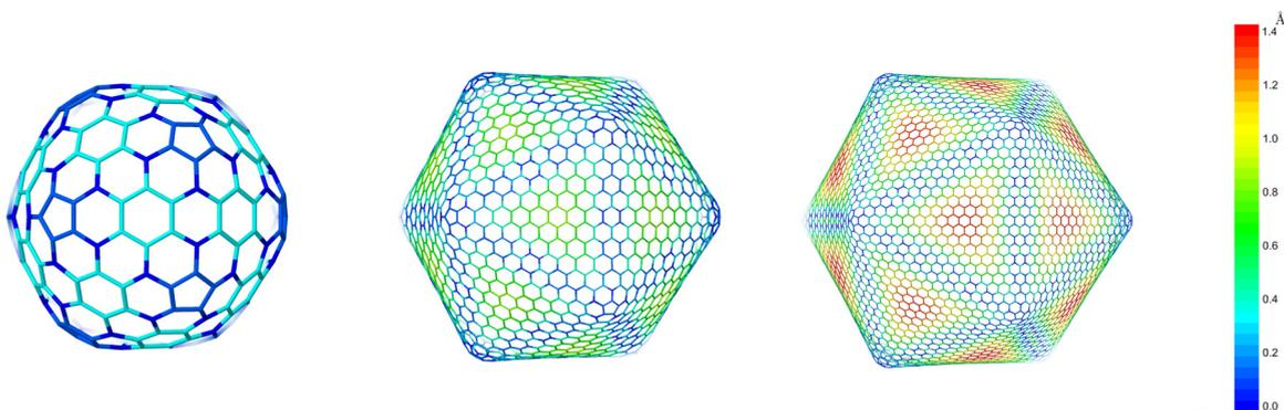
FIG. 18. Fullerenes of increasing generation-number demonstrate the polyhedral faceting transition, with  $n_{\text{full}} = 2, 6, \text{ and } 10$  structures shown in the plot (from left to right). The color scheme quantifies the displacements in atomic positions with respect to an ideally flat graphene triangle (see Ref. [7] for more details). The image is reproduced from Ref. [7], with permission from the PCCP Owner Societies.
