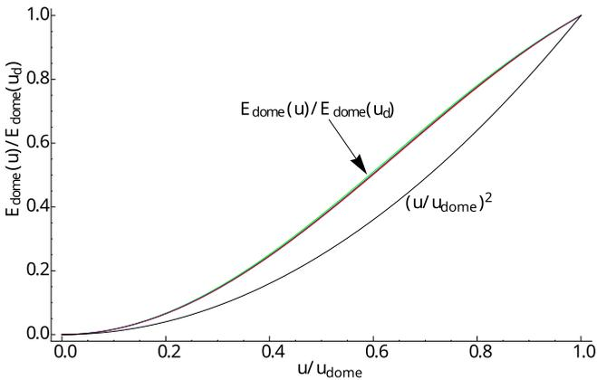
FIG. 4. Scaled in-plane strain energies of the dome given by Eq. (22) computed for  $q = \{1, 2, 3, 4, 6\}$  (almost fully superimposing curves of different colors), collapse onto a single universal curve. The values of  $A_q$  from Table I were used here. The quadratic law for the bottom curve is Eq. (25), illustrating a rather close agreement with the exact result (22).
