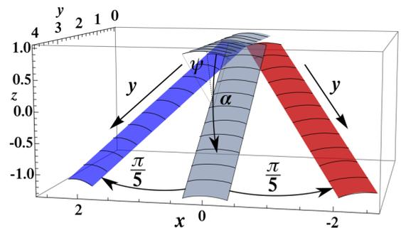
FIG. 7. Construction of the  $n = 0$  (blue) and  $n = 1$  (red) cylindrical segments for  $q = 1$  defect with the maximal tubular angle. The slope angle  $\alpha(q = 1)$  is given by  $\arccos[\sin(\pi/6)/\sin(\pi/5)]$ .
