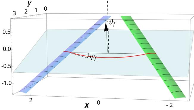
FIG. 8. Two cylindrical segments forming the edges of a variable cone. The blue inclined plane contains the bases of the arcs tilted by an angle  $\theta_{\text{face}}$ . The face angle  $\theta_{\text{face}}$  is denoted as well [see Eq. (56) for details].
