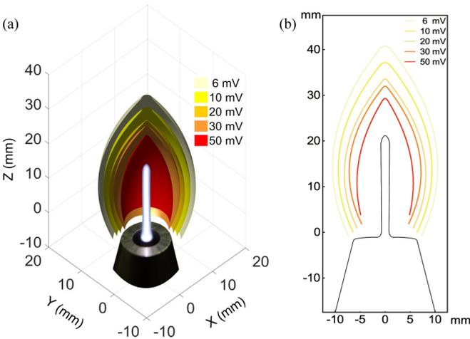
FIG. 6. Measured potential distribution around the MPJ. (a) Three-dimensional equipotential surface of potential. (b) Corresponding two-dimensional equipotential line of potential.
