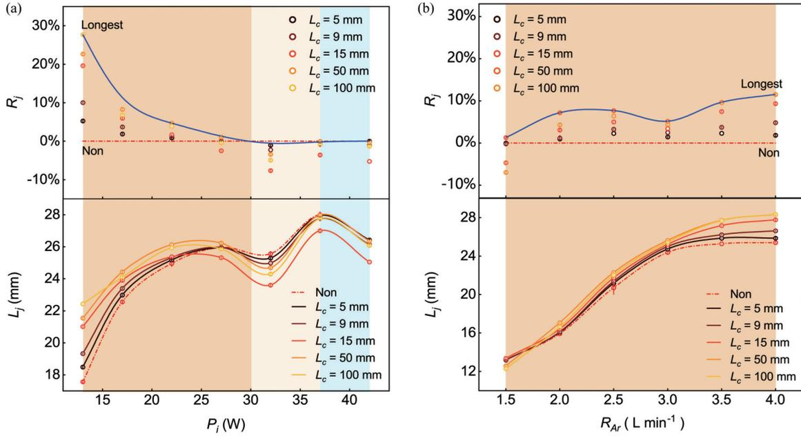
FIG. 5. The influence of microwave input power and input flow on MPJ when the nearby conductor contacts the outer conductor of the plasma generator. (a) The influence of  $P_i$  on MPJ length with different  $L_c$  when  $R_{Ar} = 3.151/\text{min}^{-1}$ . (b) The influence of  $R_{Ar}$  on MPJ length with different  $L_c$  when  $P_i = 17.2 \text{ W}$ . Data are connected by modified Bezier curves. Error bars represent the standard deviation of the measurements.
