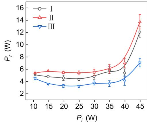
FIG. 4. The influence of nearby conductors on the microwave reflection power  $P_r$  of the system. I, II, and III represent the same cases as those in Fig. 2. Data are connected by B-spline curves. Error bars represent the standard deviation of the measurements.
