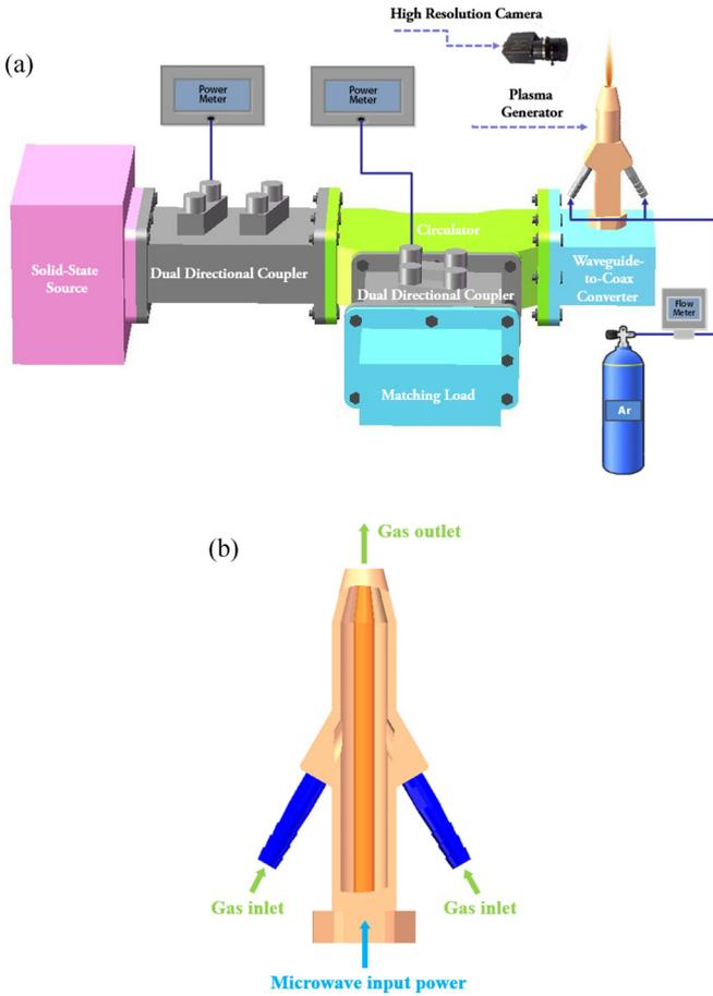
FIG. 1. (a) Schematic of the experimental system. (b) The coaxial plasma generator.
