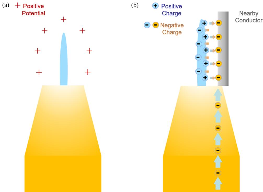
FIG. 7. Schematic of phenomena mechanism. (a) Case with no nearby conductor. (b) Case with a nearby conductor contacting the external conductor of the plasma generator.
