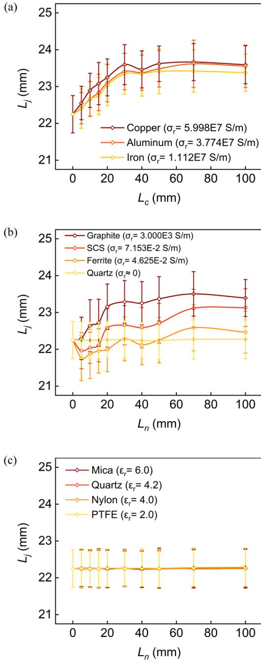
FIG. 3. The influence of nearby conductors and dielectrics with different lengths, conductivity, and relative permittivity on MPJ. (a) MPJ lengths with different metals. (b) MPJ lengths with different conductivity of nonmetals. (c) MPJ lengths with different relative permittivity of nonmetals. Data are connected by B-spline curves. Error bars represent the standard deviation of the measurements.
